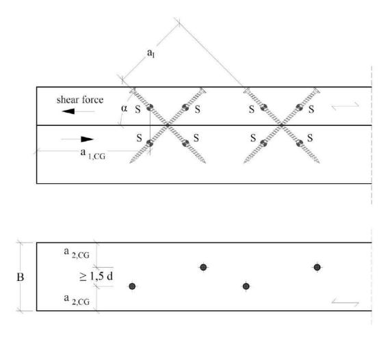
$$\begin{array}{ll} a_1 \geq 5 \cdot d \\ a_2 \geq 1, 5 \cdot d \\ a_{3,c} \geq 10 \cdot d \\ a_{4,c} \geq 4 \cdot d \end{array} \qquad \text{if } a_1 \cdot a_2 \geq 25 \cdot d^2$$
