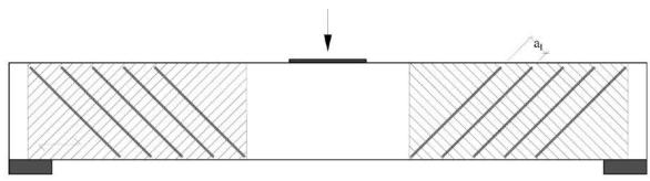
Figure E.1: Timber member with shear reinforcement; shaded areas: reinforced areas with screws arranged under  $45^{\circ}$
