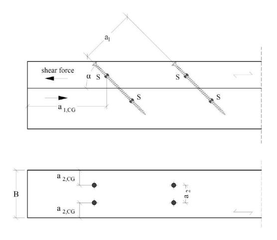
$$\begin{array}{ll} a_1 \geq 5 \cdot d \\ a_2 \geq 2, 5 \cdot d \\ a_{3,c} \geq 10 \cdot d \\ a_{4,c} \geq 4 \cdot d \end{array} \qquad \begin{array}{ll} \text{if } a_1 \cdot a_2 \geq 25 \cdot d^2 \end{array}$$
