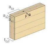
Table B1: Minimum spacing, end and edge distances of screws or threaded rods in the plane or edge surfaces of cross laminated timber
